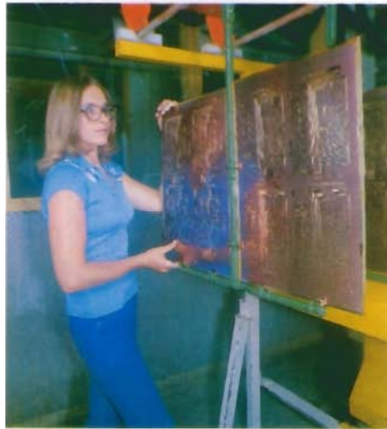
Worker loads PC boards into rack for automated plating.
